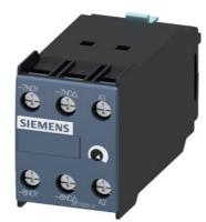
Solid-state time-delayed auxiliary switch, can be snapped on at the front, time range 1.5...30s, 100 ... 127 V AC, 2 NO, star-delta (wye-delta) function, sizes S6...S12
