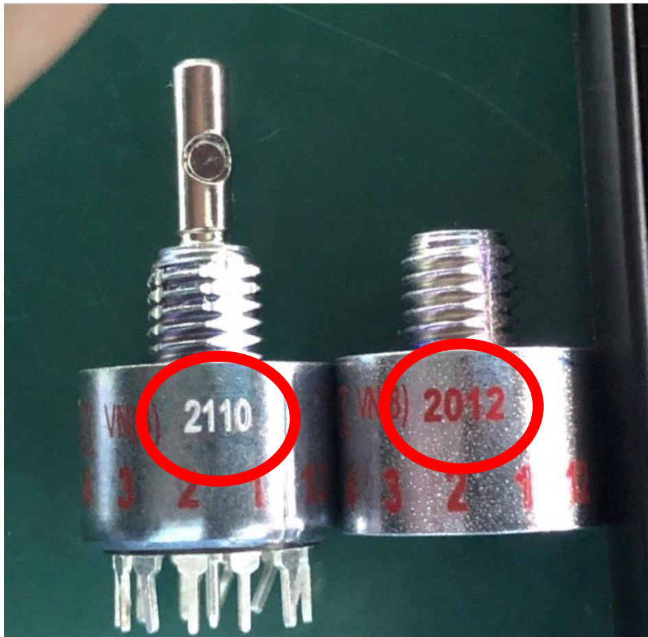
Figure 1: Comparison of Laser-marked Date Code (New, Left, Grey) vs. Print-screened (Old, Right, Red)
